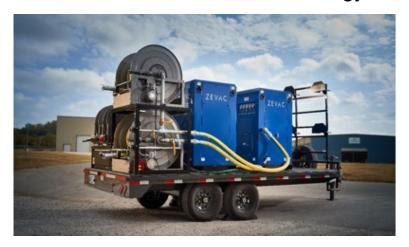
Use of ZEVAC equipment avoids methane release when replacing gas mains
